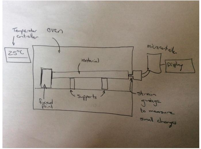
The test piece could be put in the oven and set up a 25 degrees. At the end of the material we could connect a strain gauge to measure very small movements which could be read by a microcontroller. The temperature controller can then be used to increase the temperature by 100 degrees to 125 degrees.
