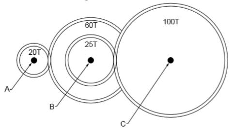
If shaft A rotates at 360 rpm, calculate the speed of rotation of shaft B and shaft C. [2 X 2 marks]
