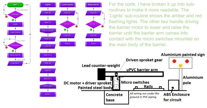
The barrier will use a large DC motor with a low-ratio gearbox to ensure there is enough torque available to raise and lower the barrier. I'd use a spline in the barrier arm to ensure it doesn't slip, and M6 threaded bar with Nyloc nuts to fasten everything together for future maintenance. By using hollow uPVC, the weight of the barrier is reduced. The lead counter-weight will balance the arm, reducing the load on the motor.
