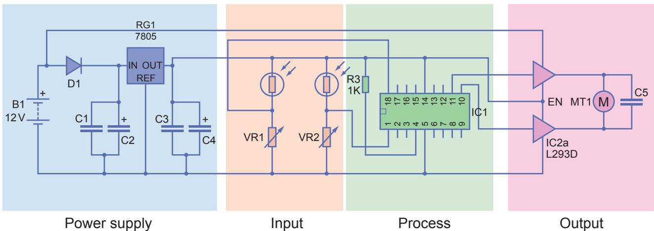
**Fig. 8** – Microcontroller circuit
