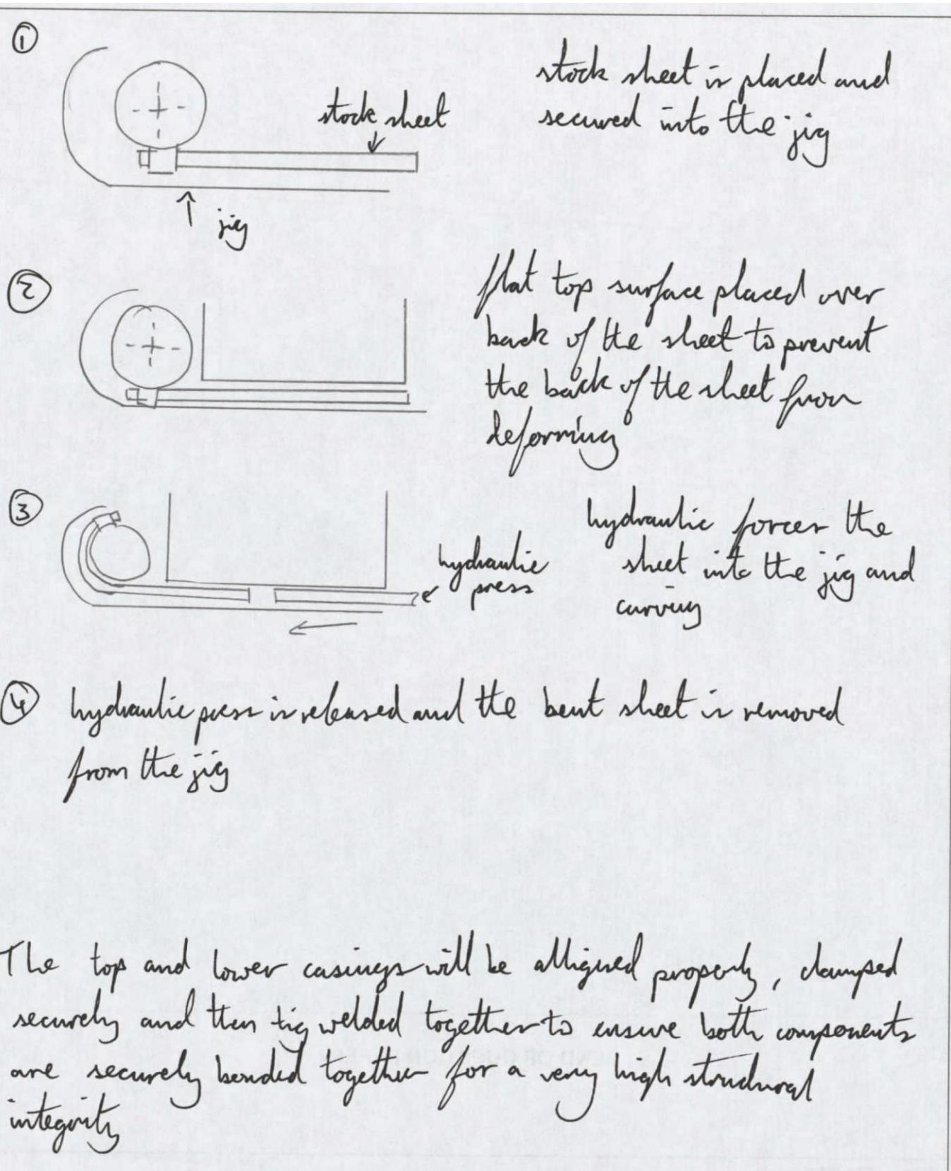
Exemplar 3 shows a Level 4 response. In this response the candidate has identified the production processes and clearly shown a good understanding through annotated sketches. All aspects of the component have been covered.
