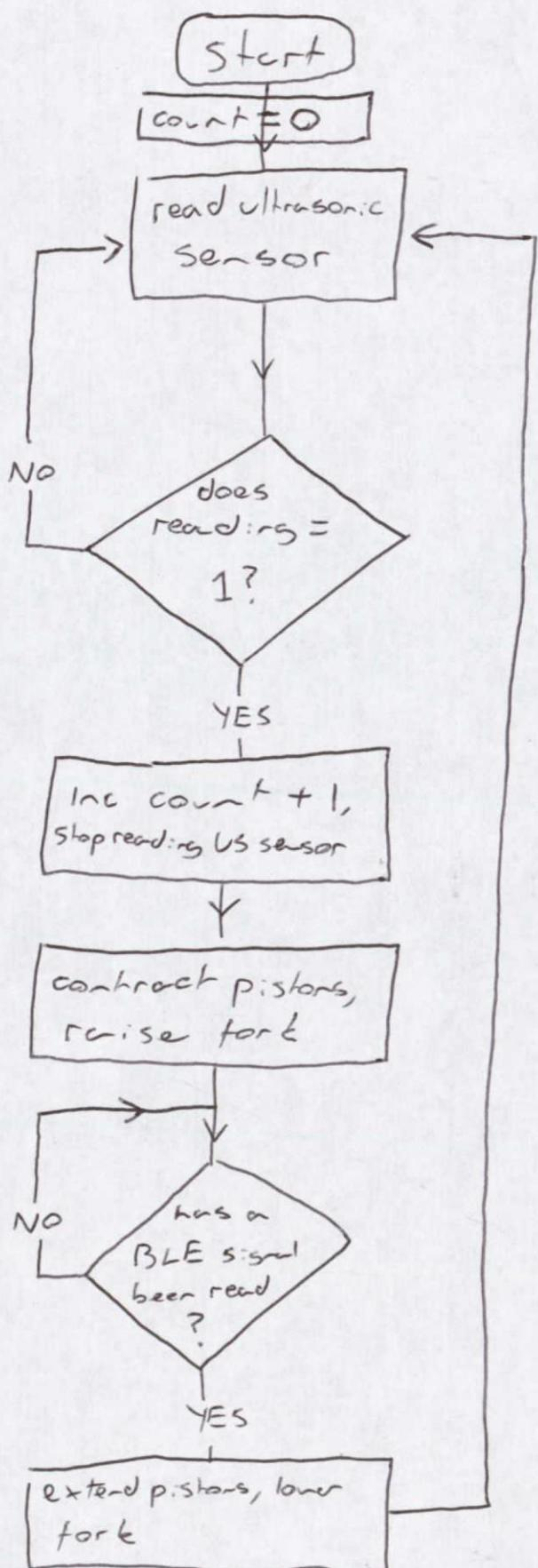
ADC:if distance  $\geq$  150, read 1if distance  $\leq$  150, read 0Buttonwhen the button is pressed assume signal sent by BLE.
