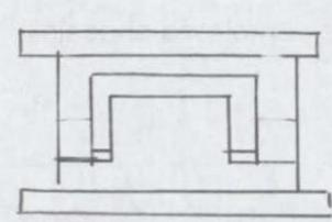
hydraulic press then clamps the dies together, bending the stamped sheet
